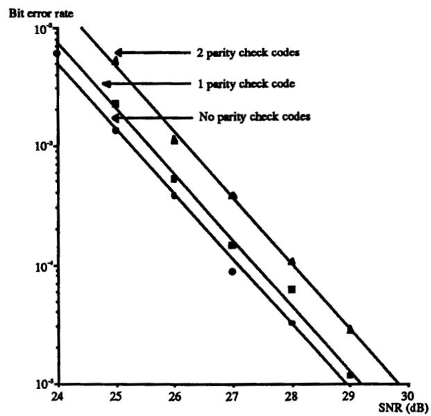
Figure 4. Performance of coding schemes over 2 PCM codec pairs.
