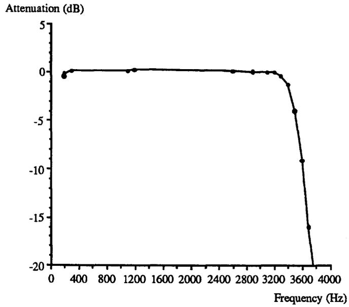
Figure 1. Amplitude response of 1 PCM codec pair.
