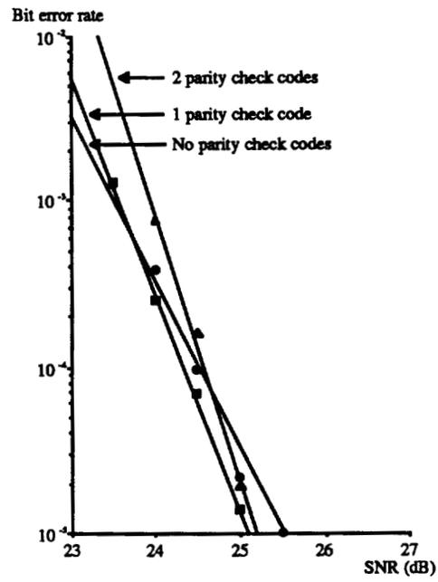
Figure 3. Performance of coding schemes over 1 PCM codec pair.
