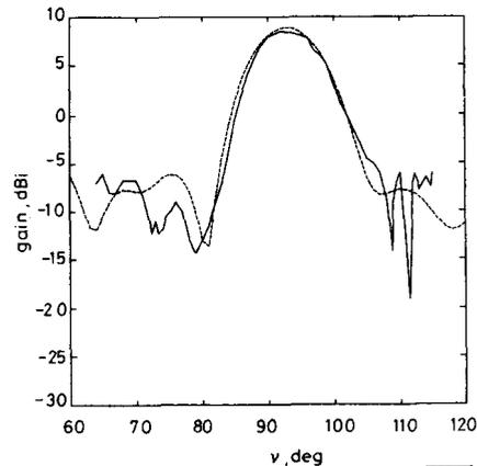
Fig. 3 Theoretical and experimental vertical pattern of dual reflector antenna
